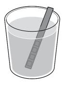
the test strip is only valid for one measurement.
