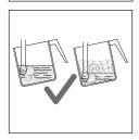
5 For proper milk foaming, keep the steam nozzle in contact with the milk and not with milk foam. Then, as the foam layer increases, slightly raise the jug keeping the nozzle in contact with the milk and without touching the bottom of the jug.
