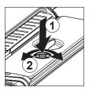
**4** Adjust the coffee grinding with the machine in operation, by pressing and turning the knob left- or rightwards of one notch at a time.
