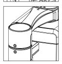
**Warning**: the carafe dispensing spout is to be tightly closed and aligned with the handle to prevent water/steam splashing or puffing.
