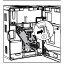
**4** Press the PUSH lever (1) and pull the handle of the brew group (2) to remove it from the machine.
