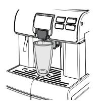
Before brewing any product and/or when bringing the dispensing spout back to its normal position, ensure that it is correctly positioned. This can be evidenced by the CLICK indicating correct positioning.
