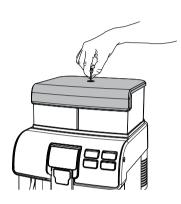
After unlocking the lid, lift and remove it.
