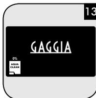
**EN** Replace the AQUACLEAN water filter with a new one.
