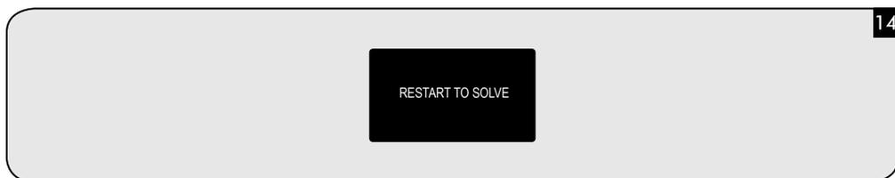
**EN** An event has occurred which requires the machine to be restarted. Take note of the code (E xx) shown at the bottom. Switch off the machine, wait 30 seconds and then switch it on again. If the problem persists, visit [www.gaggia.com/n-m-co/espesso/world-wide](http://www.gaggia.com/n-m-co/espesso/world-wide) or [www.gaggia.it/n-m-co/espesso/contact](http://www.gaggia.it/n-m-co/espesso/contact).
