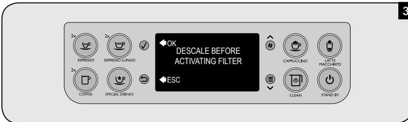
**3** Note: after replacing 8 filters, you need to descale the machine. Please refer to the "Descaling" chapter.
