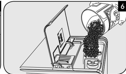
**EN** Slowly pour coffee beans into the hopper. Put the inner lid back and close the outer one.
