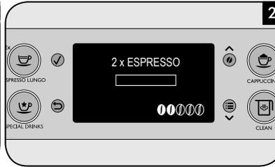
**EN** Brewing two cups of products requires two grinding and brewing cycles, automatically carried out by the machine.
