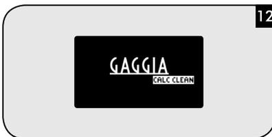
**EN** The machine needs to be descaled. Go to the Maintenance menu to select and start the cycle.
