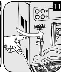
**EN** Fill with fresh water up to the MAX level.
