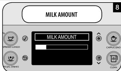
**8** By adjusting the bar on the display with the  $\blacktriangledown$  or  $\blacktriangle$  scrolling button, you can choose the amount of milk to be used for the selected beverage. Press  $\checkmark$  to confirm the change.
