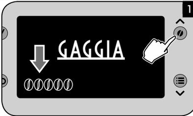
Press the button to temporarily change the quantity of coffee to grind, or to select the pre-ground coffee function.
