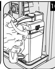
**EN** Close the milk carafe dispensing spout by turning it counter-clockwise.
