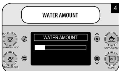
EN By adjusting the bar on the display with the or scrolling button, you can choose the amount of water used for coffee brewing.
