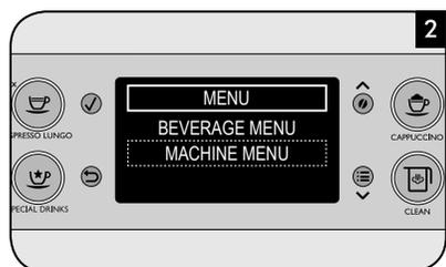
**2** Press the button to select "MACHINE MENU"; press the button to access the menu.
